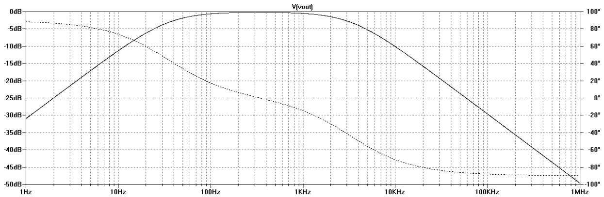
Figure 20. Characteristic of the Second Stage of the Filter
