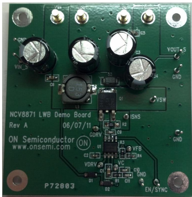
Figure 1. NCV8871LVB Evaluation Board
