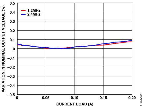
Figure 6. Inverting Regulator Load Regulation,  $V_{IN} = 5\text{ V}$ ,  $V_{NEG} = -15\text{ V}$
