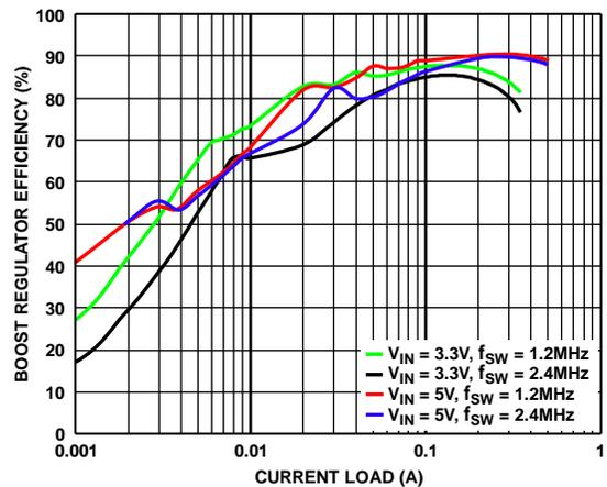
Figure 7. Boost Regulator Efficiency vs. Load Current,  $V_{POS} = 15\text{ V}$ ,  $T_A = 25^\circ\text{C}$
