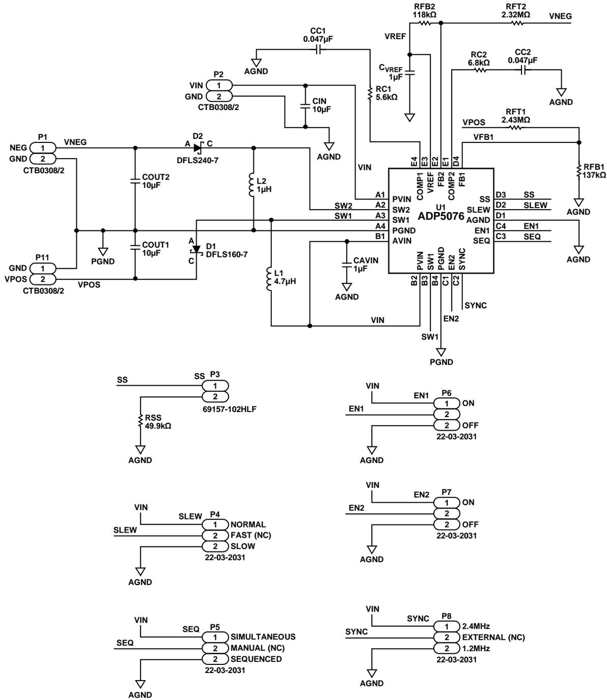
Figure 9. Evaluation Board Schematic for the ADP5076CB-EVALZ
