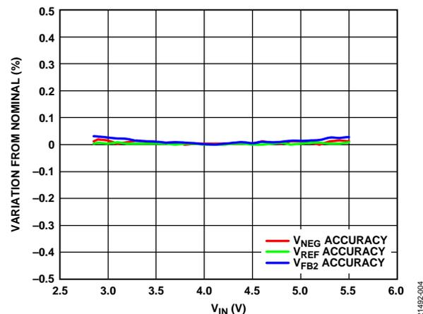
Figure 4. Inverting Regulator Line Regulation,  $V_{NEG} = -15\text{ V}$ ,  $f_{SW} = 1.2\text{ MHz}$ , 15 mA Load,  $T_A = 25^\circ\text{C}$
