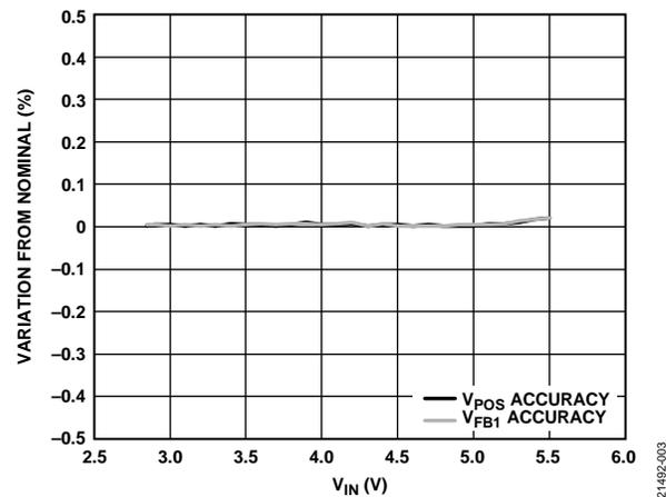
Figure 3. Boost Regulator Line Regulation,  $V_{POS} = 15\text{ V}$ , Switching Frequency ( $f_{SW}$ ) = 1.2 MHz, 15 mA Load,  $T_A = 25^\circ\text{C}$
