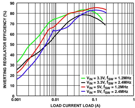
Figure 8. Inverting Regulator Efficiency vs. Load Current,  $V_{NEG} = -15\text{ V}$ ,  $T_A = 25^\circ\text{C}$
