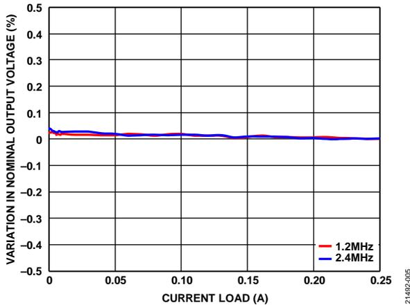
Figure 5. Boost Regulator Load Regulation, Input Supply Voltage Range ( $V_{IN} = 5\text{ V}$ ,  $V_{POS} = 15\text{ V}$ )
