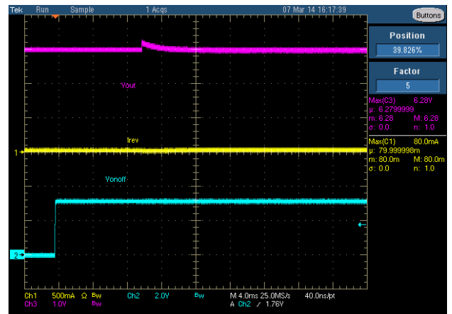
Figure 57. Prebias Waveform (CH1: Reverse Current; CH3: Output Voltage) at 36 V Prebias Soft Start from 6.0 V (0xFE6C[1] = 1, 0xFE39 = 58h)
