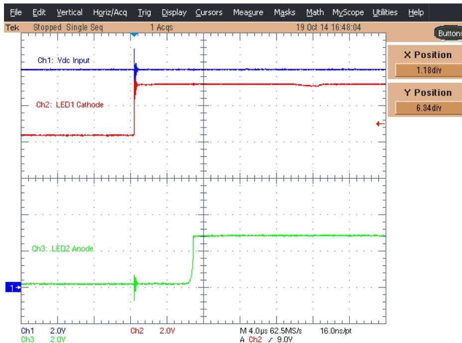
Figure 3: LED1 short circuit failure. LED2 turns on about 7 \mu s after LED1 fails.
